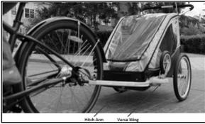
through July 2010) located on the left side of the frame. Recalled conversion kits have hitch arms that attach the carrier to the bicycle with model number "20100503"
